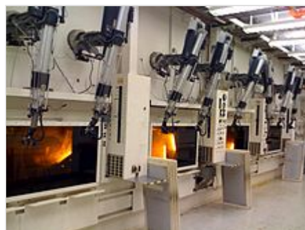
Most waste packaging, small-scale experimental fuel recycling chemistry and radiopharmaceutical refinement is conducted within remote-handled hot cells .
